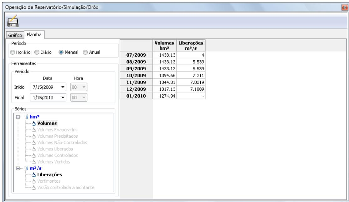
Figure 2: Storage and release results for the Oros reservoir using the priority simulator in SIGA and inflow zero after the rainy season.
